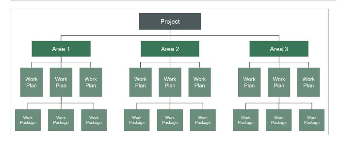
As mentioned in the scenario above, the scope of the Steel Structure project was too big to manage without segmenting it down to work packages representing one to four weeks' worth of work. In Plan, this breakdown of the project could look like this:
