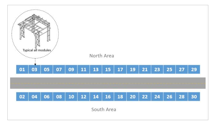
Using the scenario above as an example, assume that you initially break the project into two construction work areas (CWA): North Area and South Area. You break each area of work into three different construction work packages: Earthwork, Foundation, and Steel Erection. From there, you can
